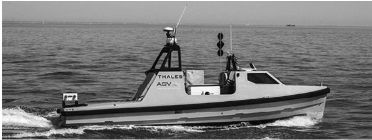
Figure 12: Thales Halcyon USV used in decoy experiments
