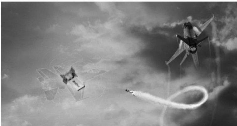
Figure 14: BriteCloud decoy simulating a defended aircraft
