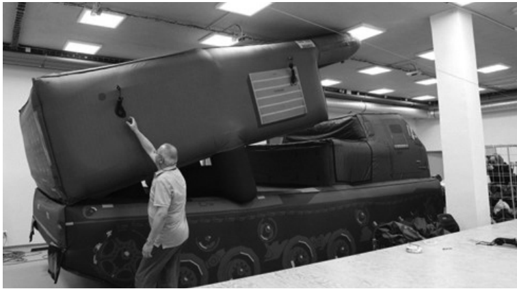
Figure 15: Inflatable decoy High-Mobility Artillery Rocket System (HiMARS) 55
