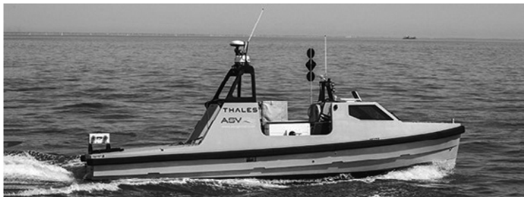
Figure 12: Thales Halcyon USV used in decoy experiments
