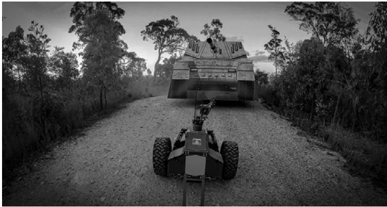
Figure 17: The Raider Targetry Mobile Moving Target System, which combines an uncrewed ground vehicle with a rigid target
