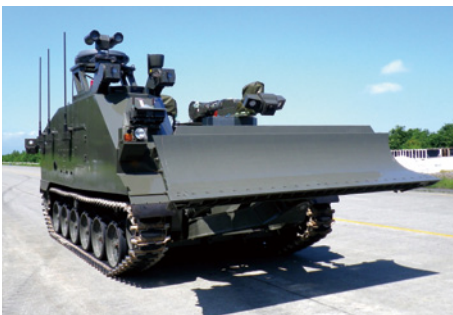
Remote-controlled small reconnaissance vehicle system (Japan Ministry of Defense)
